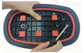
3. Replace the filter and push the rubber plug to secure the filter.
